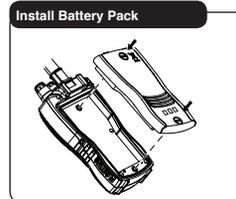
When your rechargeable batteries begin to discharge too quickly, it is time to install a new battery pack. Your radio will also operate with five (5) high-quality AA alkaline batteries, using the included alkaline battery tray.
